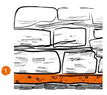
Foundation consisting of an approx. 40 cm high layer of sand and gravel, which is tamped and compacted (not necessary if the subsoil is highly compacted). Foundation stones are embedded into the ground.
