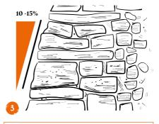
Place the bricks accurately, place through stones regularly, and carefully layer the backing stones. Keep to an incline of 10-15 %.
